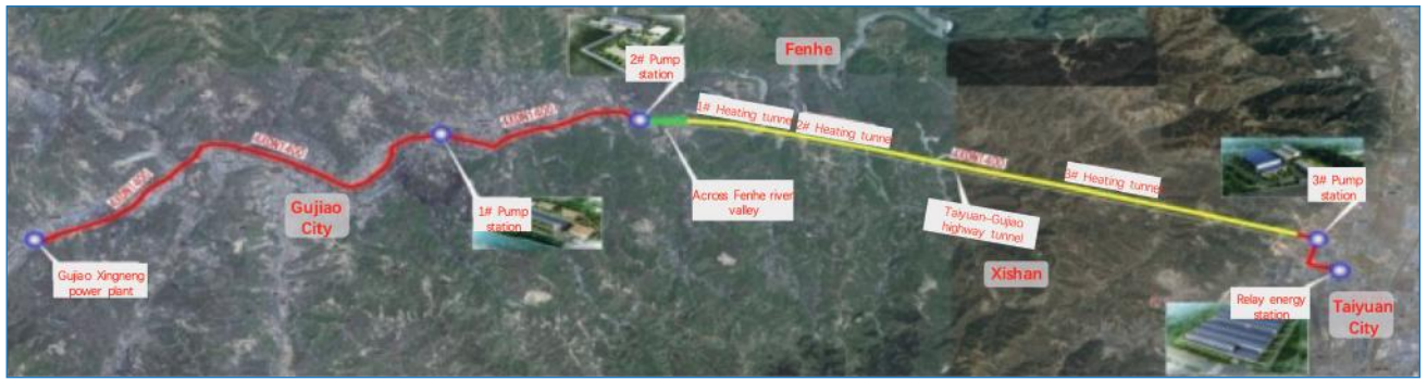
Fig. 2.14. General layout of the main heating pipeline from the Gujiao power plant to Taiyuan
